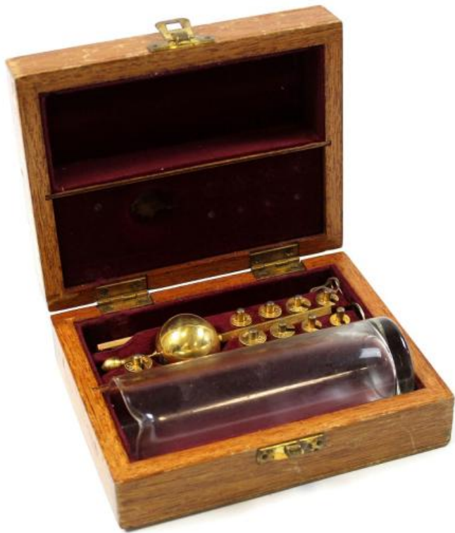
1356 Cased hydrometer set with ivory rule in fitted case by Peter Stevenson Ltd. Presented in a fitted case with all weights present.
